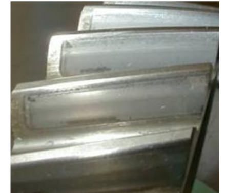
Gear micro-pitting failure
