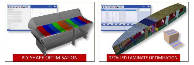
**Ply Shape Optimisation** – The technique, developed through OptiAssist's application in Formula  $1^{\text{M}}$ , allows users to automatically develop laminates based upon multiple structural requirements with the freedom to evolve the ply preforms. Users can define candidate ply materials, types and orientations and closely control the sub-division of preforms in order to achieve manufacturable solutions.
